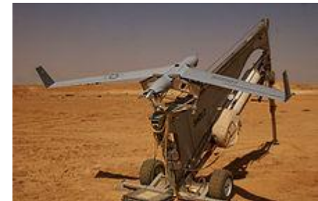
ScanEagle reconnaissance UAV on its catapult launcher
